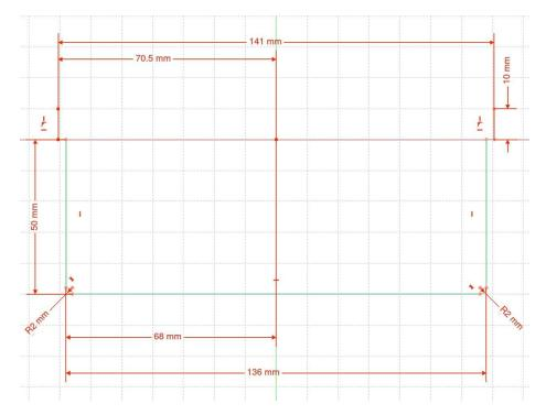
The above drawing shows the cross section of the Cansat. The 136 mm diameter is for the shoulder portion of the Cansat and is a required dimension that must be implemented. Exceeding 136 mm will can cause the Cansat to get stuck in the rocket. If the diameter is smaller, the Cansat can shift around and affect the flight direction of the rocket. Worst case, wraps of tape would be required to compensate for a smaller diameter.
