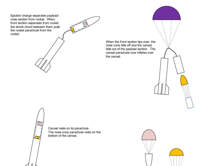
The cansat, nose cone, and rocket descend under parachutes.
