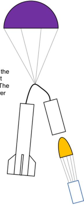
Cansat rests on its parachute. The nose cone parachute rests on the bottom of the cansat.
