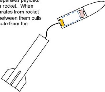
When the front section tips over, the nose cone falls off and the cansat falls out of the payload section. The cansat parachute now inflates over the cansat.
